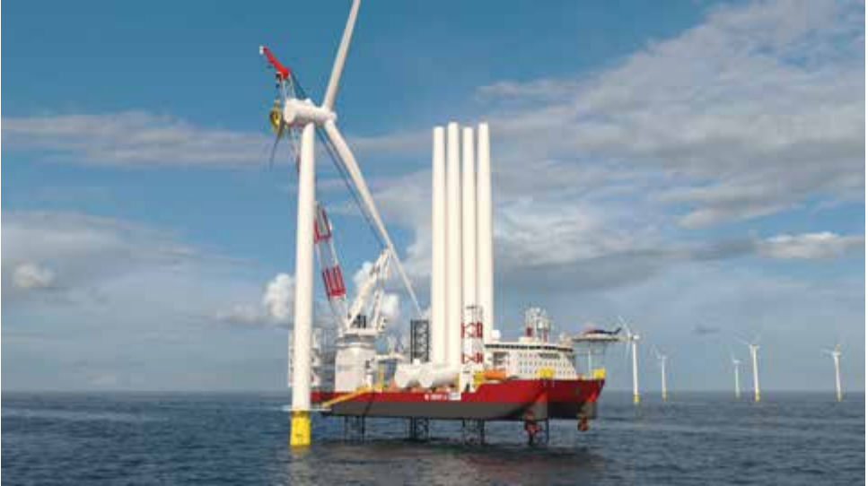
Depiction of Wind Turbine installation Vessel CHARYBDIS. Picture source: Dominion Energy.
