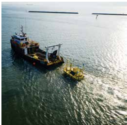
Deployment of Surface Meteorological Buoy of North Carolina Coast. Picture source: Avangrid Renewables.
